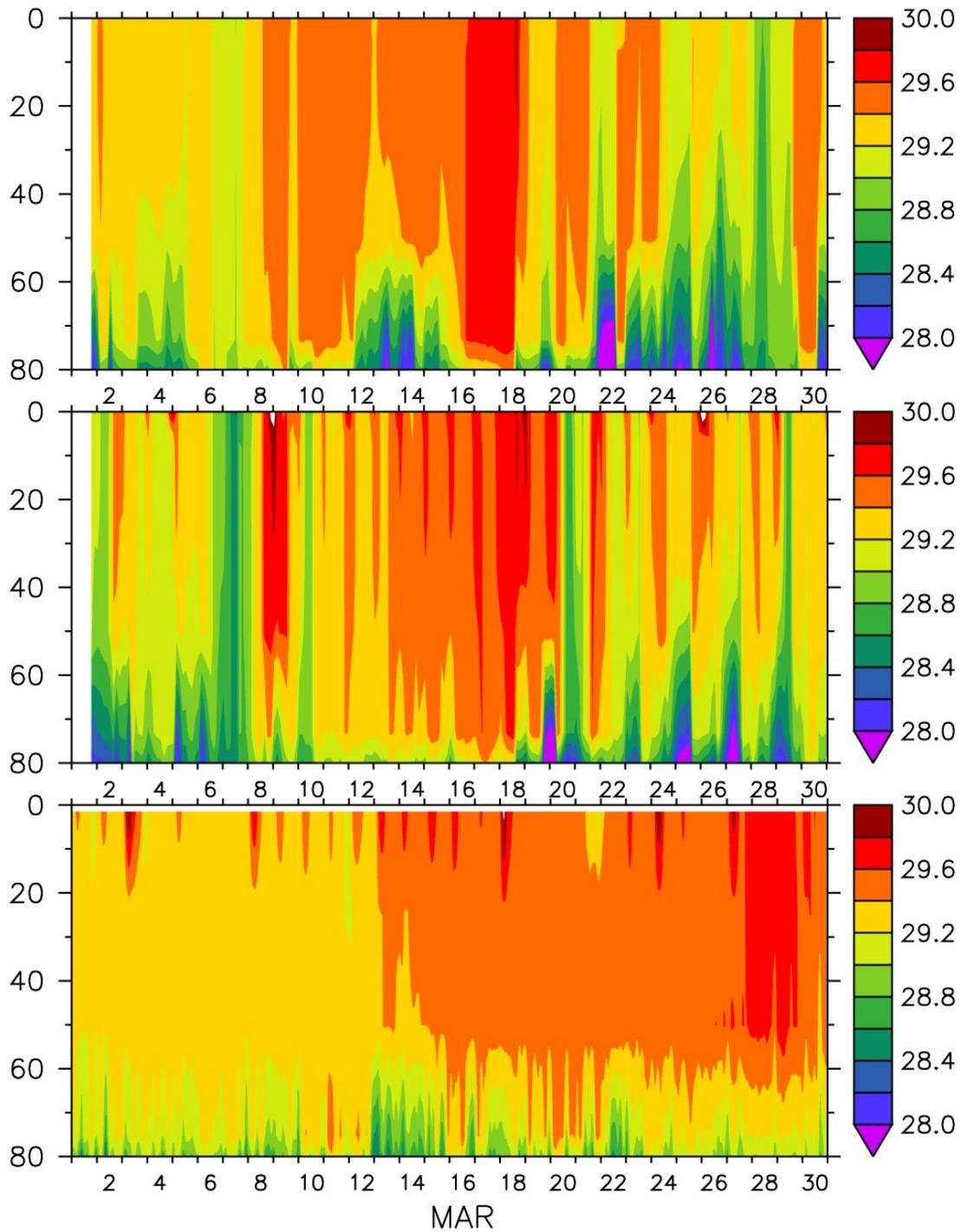
Figure 2: Temperature ( $^{\circ}\text{C}$ ) vs. depth as a function of time for March 2008 at  $137^{\circ}\text{E}$ ,  $5^{\circ}\text{N}$  for hindcast 80.4 without the diurnal cycle (top), hindcast 80.3 with the diurnal cycle (middle) and observations from a TAO buoy (bottom). The tick marks at the bottom mark the beginning of each day and the numbers are marked at the middle of the day. The GOFS V3.0 output are 3-hourly whereas the TAO observations are 1-hourly.
