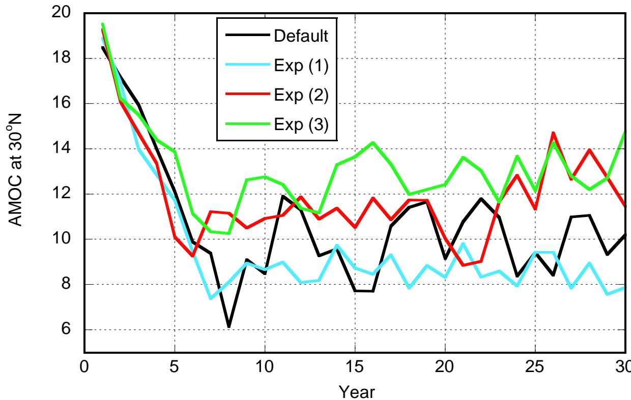
The AMOC index is the maximum overturning streamfunction in 500-3000 m at 30°N.
