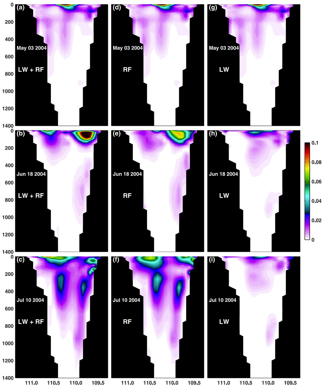
**Figure 14.** Kinetic energy snapshots (color contours in  $\text{m}^2/\text{s}^2$ ) for three different dates during spring–summer of 2004. Simulated with the  $1/12^\circ$  nested interannually forced GOC–HYCOM experiments over a cross–section at the latitude of Topolobampo. (a)–(c) Forced with local plus remote forcings, (d)–(f) forced with remote forcing only, and (g)–(i) forced with local forcing only.
