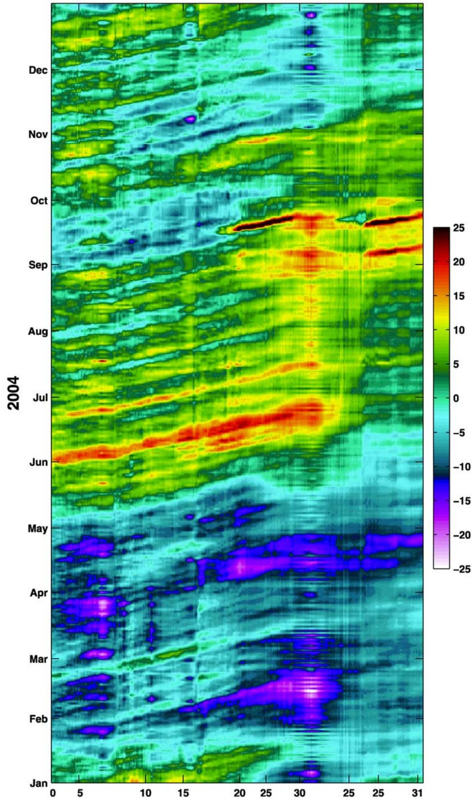
**Figure 10.** Sea surface height (in centimeters) time series for 2004 from  $1/12^\circ$  interannually global HYCOM simulation along the coast of the North American continent from  $0^\circ\text{N}$  to  $32^\circ\text{N}$  as shown in Figure 7. Latitudes along the coast are indicated, including the three times when the coastline reach the latitude of  $25^\circ\text{N}$ .
