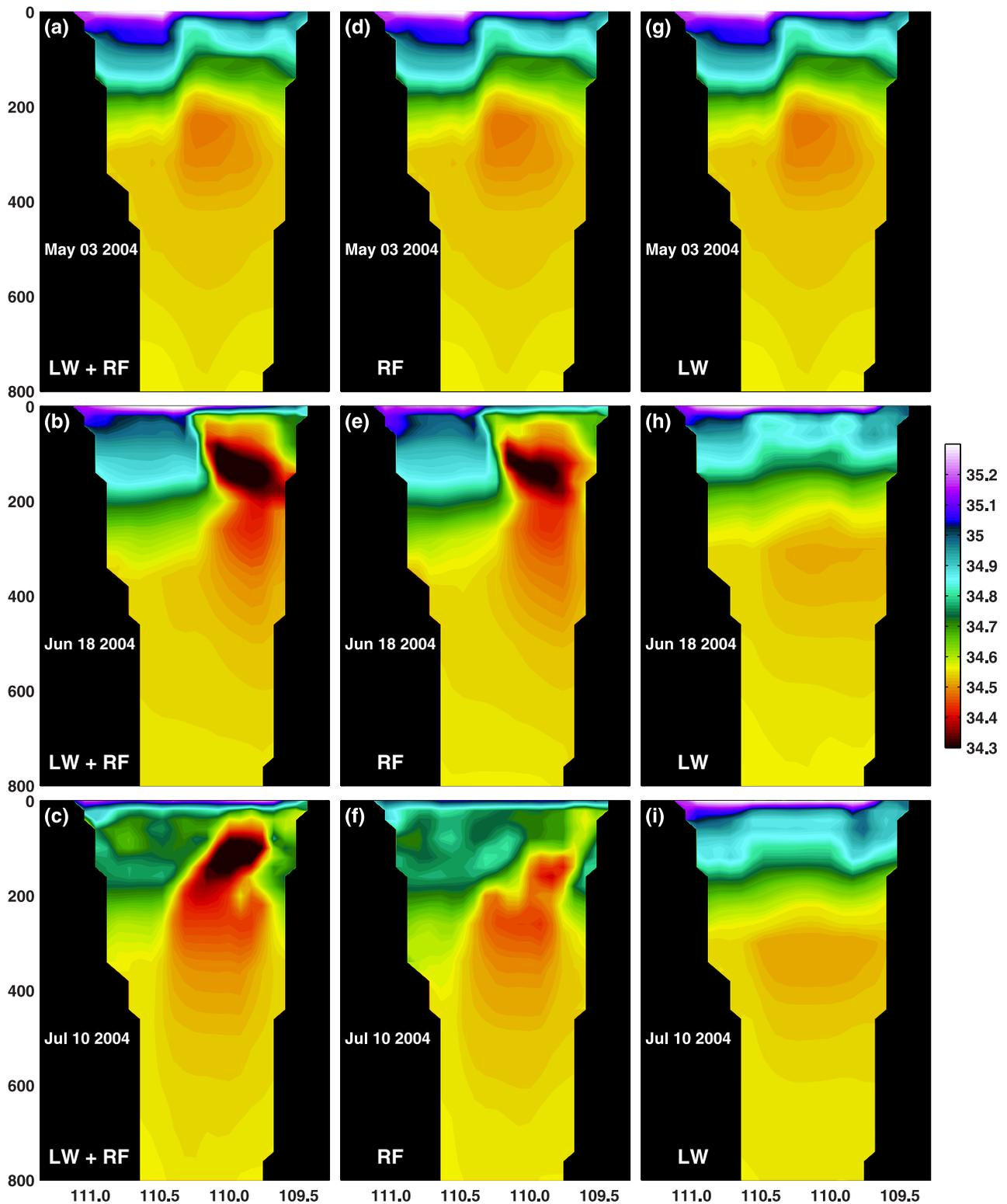
**Figure 13.** Salinity snapshots (color contours in psu) for three different dates during spring–summer of 2004. Simulated with the  $1/12^\circ$  nested interannually forced GOC–HYCOM experiments over a cross–section at the latitude of Topolobampo. (a)–(c) Forced with local plus remote forcings, (d)–(f) forced with remote forcing only, and (g)–(i) forced with local forcing only.
