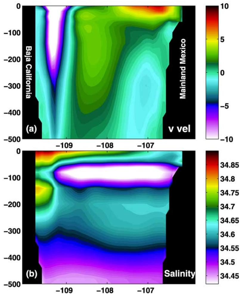
**Figure 2.** A 7-year mean of (a) meridional currents (color contours in cm/s), and (b) salinity (psu) as determined from the climatologically forced Pacific HYCOM simulation over a cross-section along a west-east line at  $\sim 23.2^\circ\text{N}$  (close to the entrance of the GOC), which has the coast of the Baja California Peninsula on the west and the coast of mainland Mexico on the east. Positive currents indicate northward flow.
