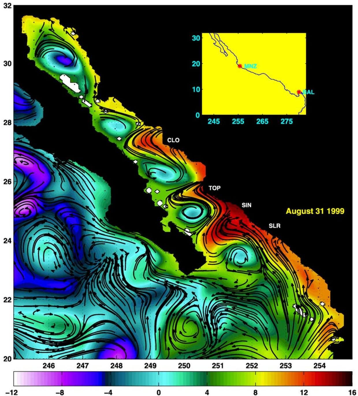
**Figure 7.** Sea surface height (color contour in cm) and top layer currents (arrow vectors) for August 31, 1999 as determined by the  $1/12^\circ$  interannually forced Pacific HYCOM simulation. The yellow insert includes the North American continent coastline from  $0^\circ\text{N}$  to  $32^\circ\text{N}$  along which the along-coastal versus time sea surface height diagrams of Figures 8 and 10 were calculated. The positions of Balboa (BAL) and Manzanillo (MNZ) are indicated.
