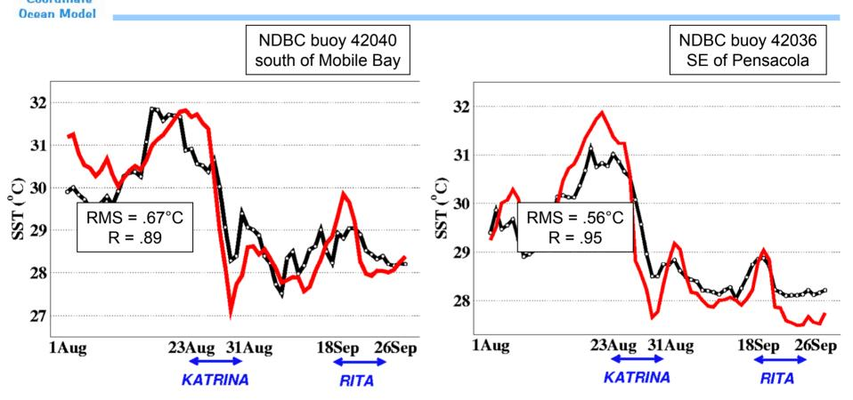
HYCOM reproduces the deterministic SST response to the wind forcing. Implies realistic upwelling and mixing of subsurface waters as well as realistic atmospheric wind and heat flux forcing.
