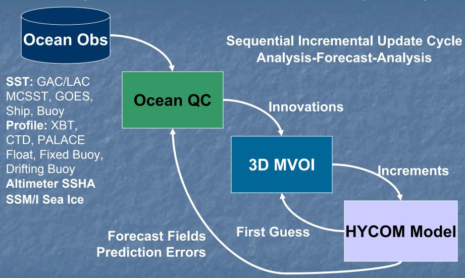
MVOI - simultaneous analysis 5 ocean variables temperature, salinity, geopotential, velocity (u,v)
